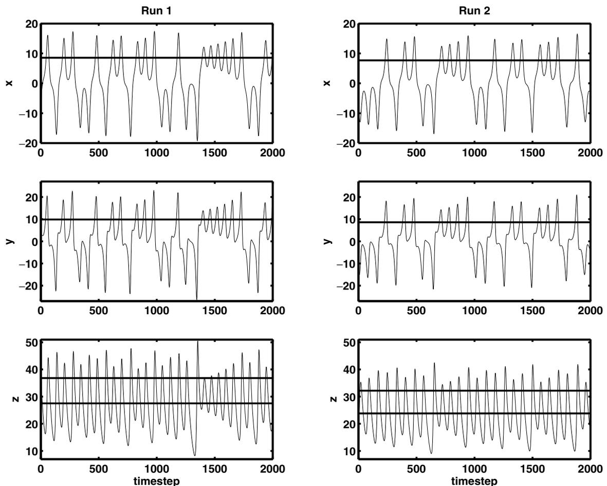
Fig. 1. Two example model runs with different parameter values. The horizontal lines indicate the climatological statistics (mean of  $z$ , and amplitude of the oscillations of all three model variables) of the model runs.
