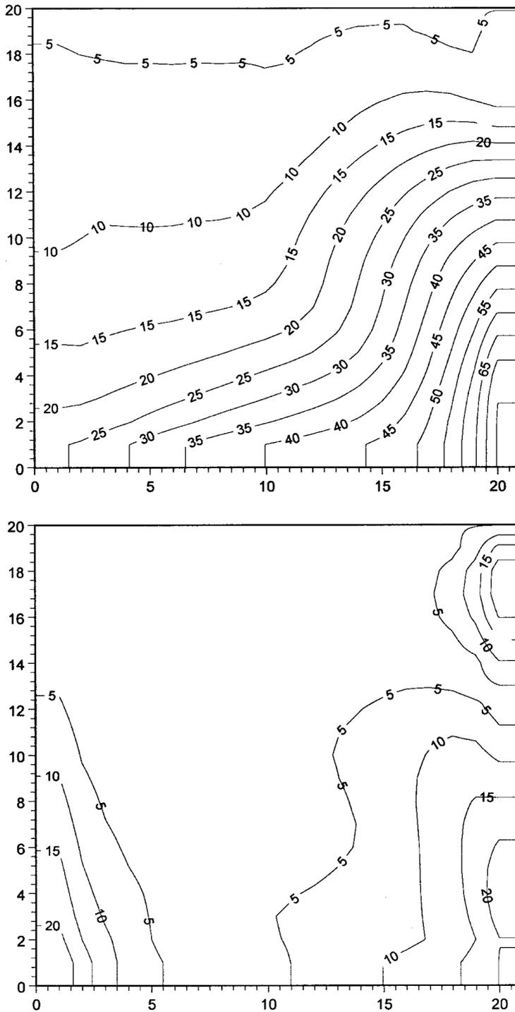
Figure 11. Spatial distribution of r.m.s.e. (cm) of the wrong model (top) and the updated model based on the EnKF (bottom).
