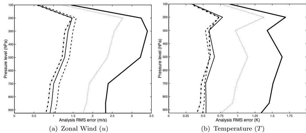
**Figure 5.** We plot the average analysis RMS error as a function of vertical model level from assimilating simulated rawinsonde observations alone (thick solid) and rawinsondes with satellite retrievals. We assimilate retrievals within the local region (dotted) and also those retrieval observations outside the local region with a correlation coefficient of at least 0.25 (dashed), 0.15 (dash-dotted), and 0.05 (thin solid).
