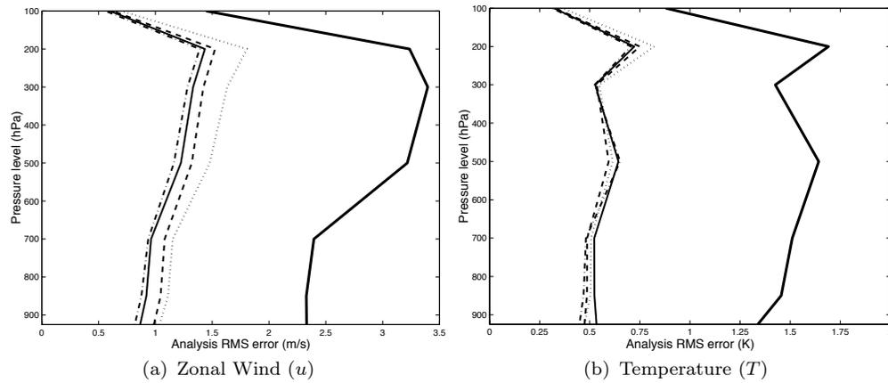
**Figure 4.** We plot the average analysis RMS error as a function of vertical model level in from assimilating simulated rawinsonde observations and satellite radiances. We select rawinsonde observations within a local region 1 level deep (thick solid) and we also assimilate the radiance observations if the value of the  $h$  operator there is greater or equal to 0.5 (dotted), 0.25 (dashed), 0.125 (dash-dotted), and 0.0625 (thin solid).
