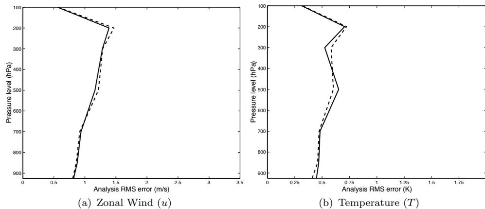
**Figure 6.** We compare the best result from assimilating the simulated rawinsonde and satellite radiance observations (solid) and the simulated rawinsonde and satellite retrieval observations (dashed) by plotting the average analysis RMS error as a function of vertical model level.
